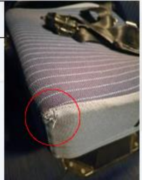
FO seat cover damaged
